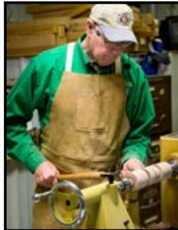
The November demonstration was done by Larry Rogers. Larry reprised a demo from 2008 or 2009. Larry's sphere making technique is an Old World method. A billet is turned to a cylinder whose diameter equals the sphere's desired size. Using a caliper, the diameter is scribed onto the cylinder.
